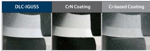
Figure 4. Wear condition of ball flank after milling 420 m.
